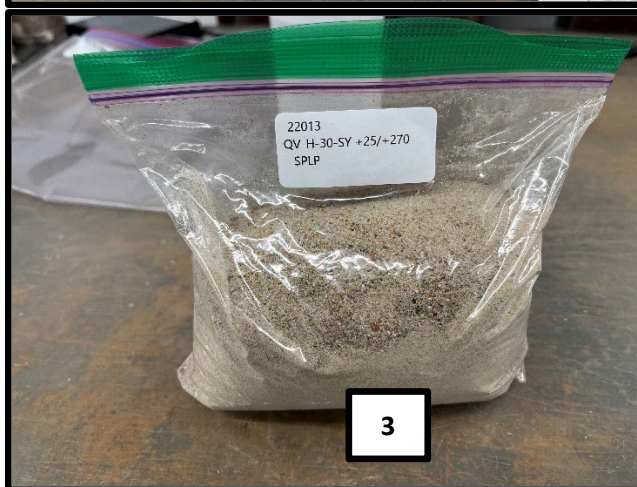
Figure 27. Illustration of Sample Splitting Process After Wet Sieve Separation
