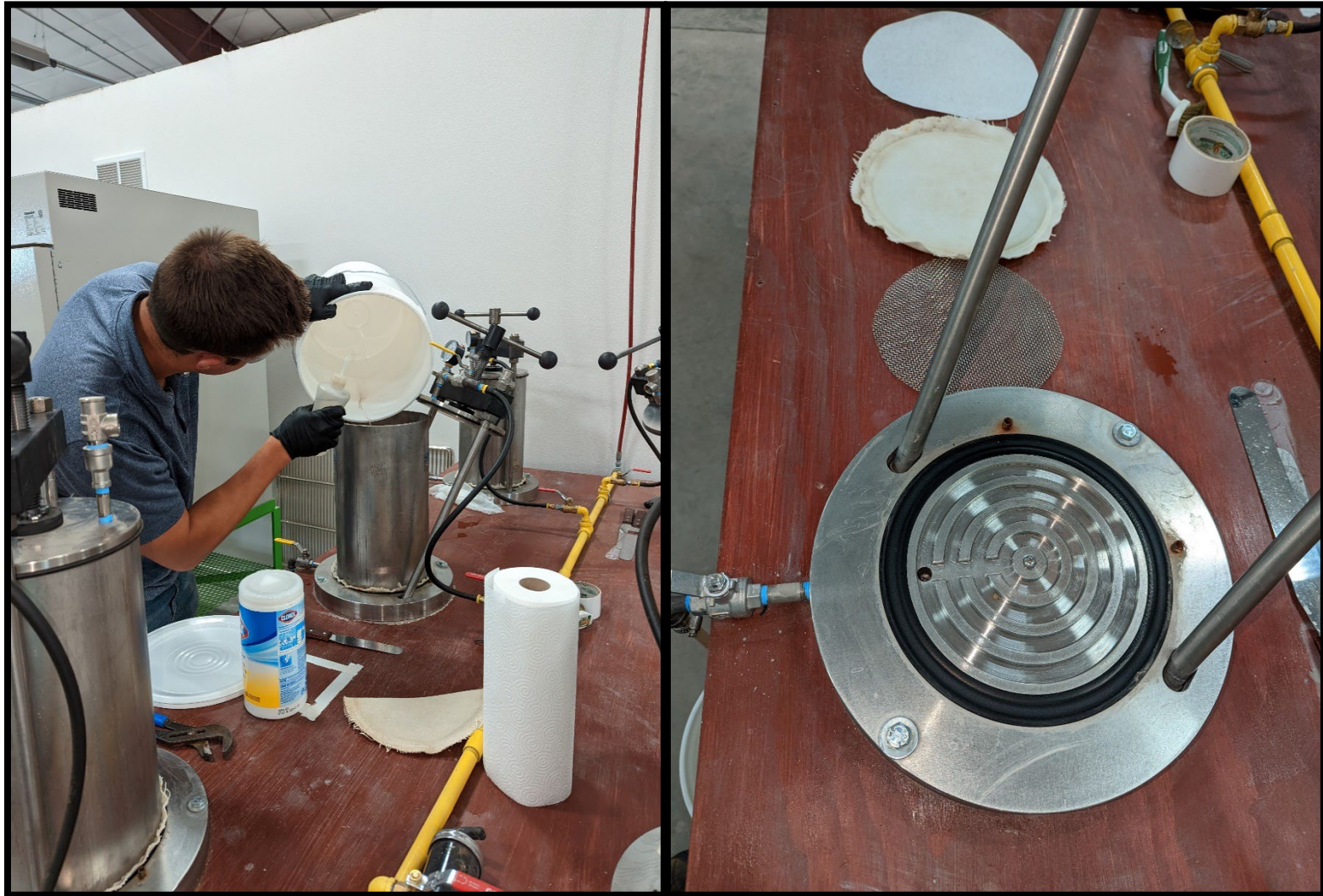
Figure 24. Pressure Filter Apparatus at the Disa Process Laboratory Used for Removing Water from the Passing 270-Mesh Fraction after Wet Sieving with All Components Laid Out on the Table
